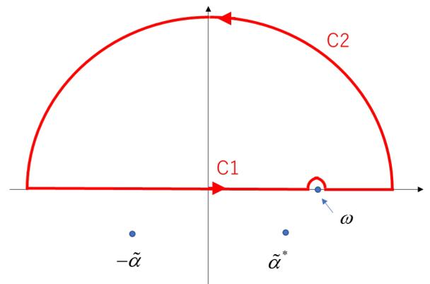
$$\oint_{C_1+C_2} \frac{\tilde{\chi}(\tilde{\Omega})}{\tilde{\Omega}-\omega} d\tilde{\Omega} = 0$$
